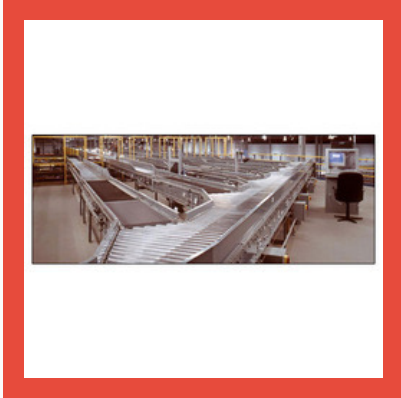
Case Handling Conveyors
