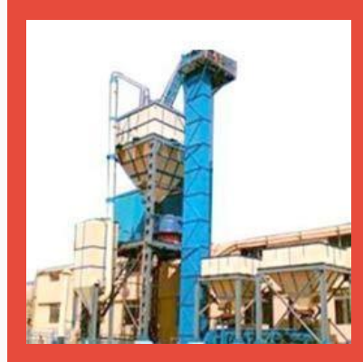
Belt Bucket Elevators
